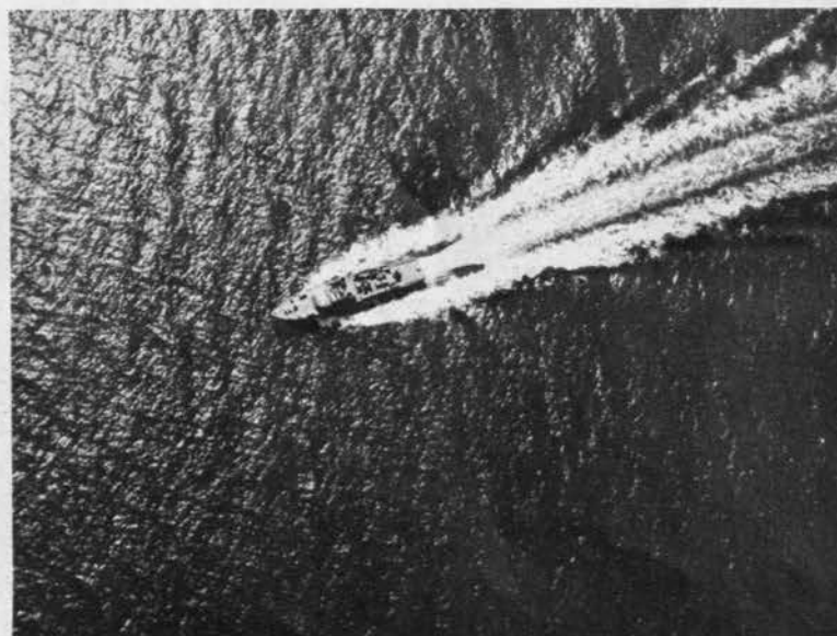
Less streamlined than the smaller picket boats, the new 104-ft. type is still a cleanly designed vessel. Note the ventilators and other gear on the afterdeck, also the U-shaped cabin with two round gun positions.
